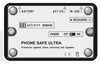
The orange, 'IN USE' LED on the right side, will indicate that a phone is installed in the device.
