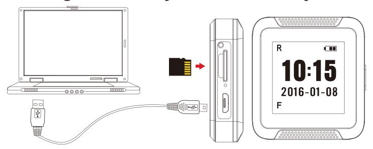
Plug the micro USB end of cable into USB port and plug the other end into the computer or other USB power source. After charging, with golden contact facing up, insert the memory card into the card slot. Then the device will be ready for further operations.
