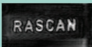
Word "RASCAN" cut from aluminum foil, under 6 cm of foamed concrete (frequency is 6.6 GHz)
